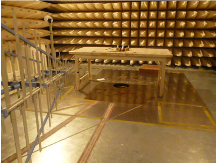
Photograph 1: Set-up for Radiated Emission
